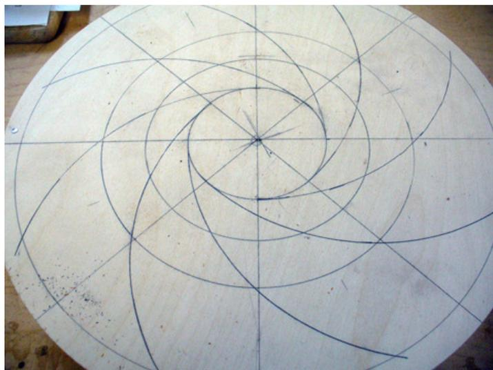
Using a plunge router with a 1/4" upcut spiral bit and a trammel base I set the pivot point the same as above when I marked it. Then, taking shallow cuts, I cut out the arcs **making sure that every second arc only went from the outside circle to the third circle in from the outside**. This would ensure that more wood for
